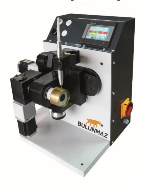
This cutting-edge device utilizes ultrasonic vibrations and a programmable logic controller (PLC) to effortlessly adorn your accessories with vibrant patterns. With its user-friendly operation and precise controls, you can easily program and automate intricate designs. Say goodbye to manual labor and hello to the future of personalized jewelry.
